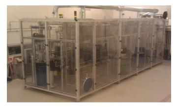
A pilot plant is a development stage in-between lab scale and commercial scale. It is a valuable development procedure that can be used to get an idea of whether or not a process is economical feasible. This pilot plant is approximately 3x3x8 m and is able to process up to 60 litres biomass slurry per hour.
